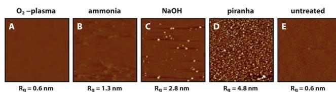
**Figure 2.** AFM pictures after surface treatments reveal differences in roughness of the surface. More stronger cleaning procedures created a rougher surface as expected.  $R_q$  is surface roughness determined by AFM. Image size is  $10 \times 10 \mu\text{m}$ .
