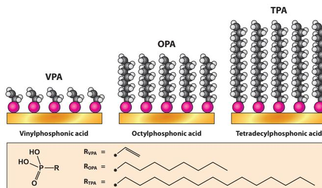
Figure 1. Various organophosphonates were measured using MP-SPR.
