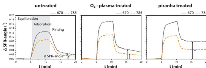
**Figure 3.** Tetradecylphosphonic acid (TPA) adsorbed only slightly onto the untreated gold surface, adsorption was slightly better to the  $\text{O}_2$  plasma and NaOH treated surfaces, however, piranha and ammonia treated surfaces were clearly more favourable for the adsorption.
