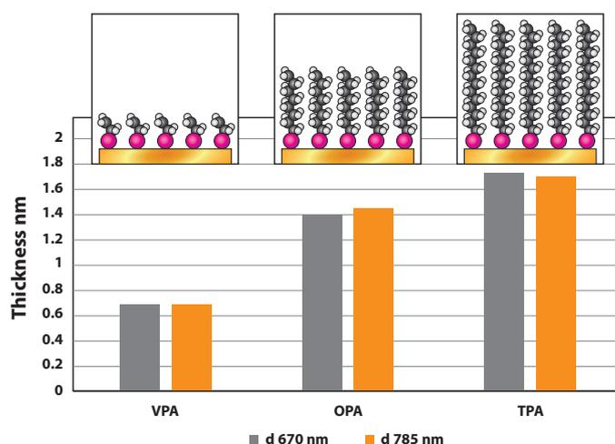
**Figure 4.** SAM thicknesses: vinylphosphonic (VPA), octylphosphonic (OPA), and tetradecylphosphonic acid (TPA).
